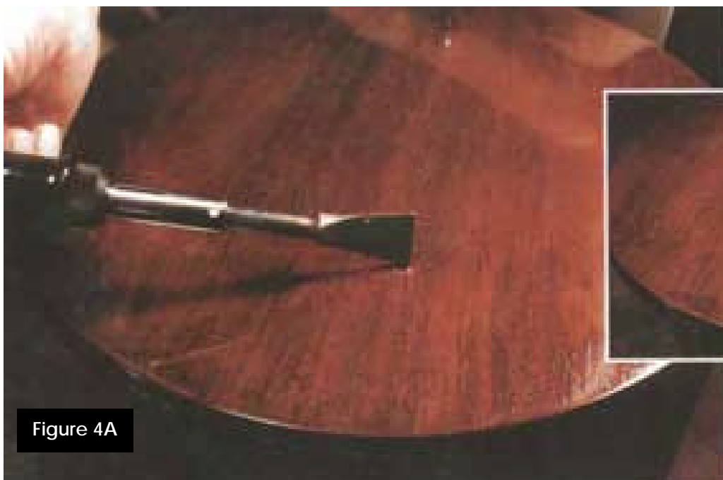
Figure 4: Fill the defect with the melted material (A) until it is slightly overfilled (B).
