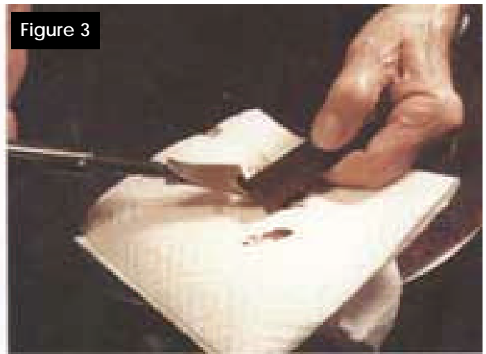
Figure 3: Melt a bit of the burn-in stick onto the tip of the knife.
