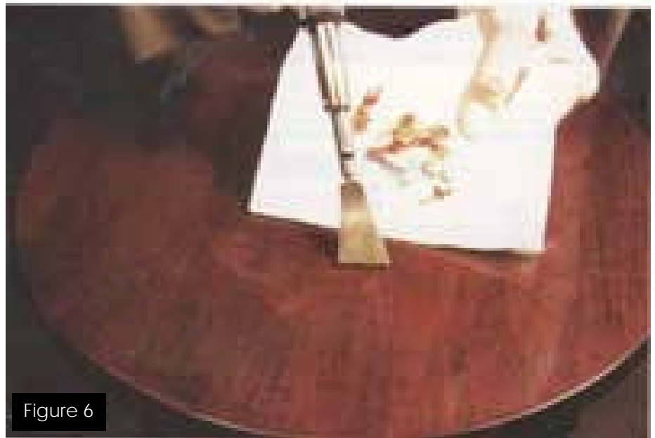
Figure 6: Gently scrape the excess fill onto the lubed area.
