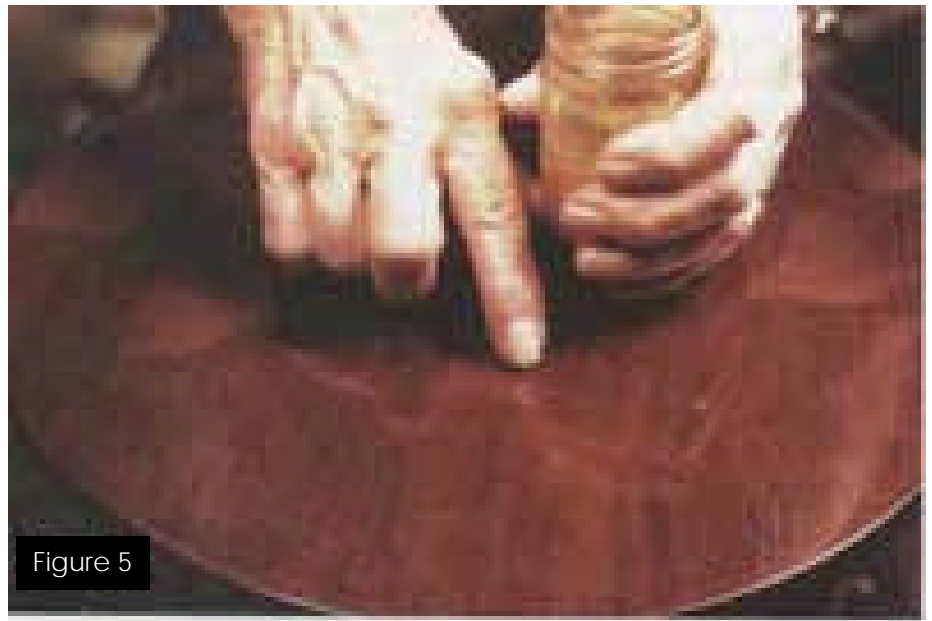
Figure 5: Apply a little patch lube on one side of the filled gouge.
